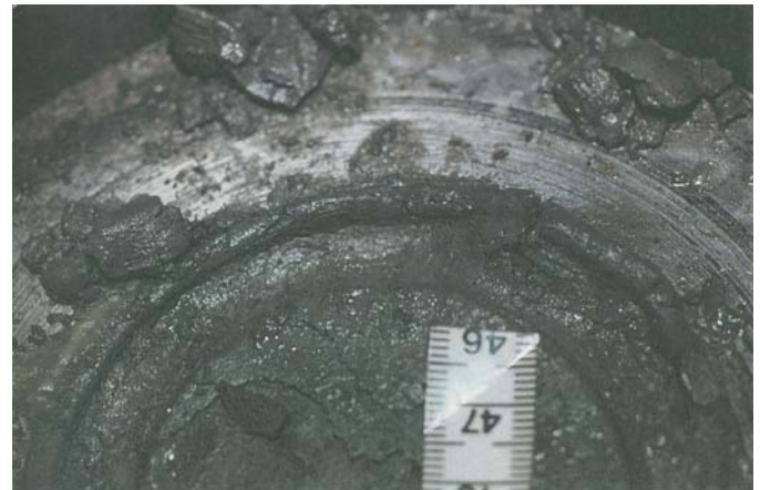
Fig. 17. Cutting ribbons from single cutter tests with interference plate in water at 9000 psi and 0.011" depth of cut 1
