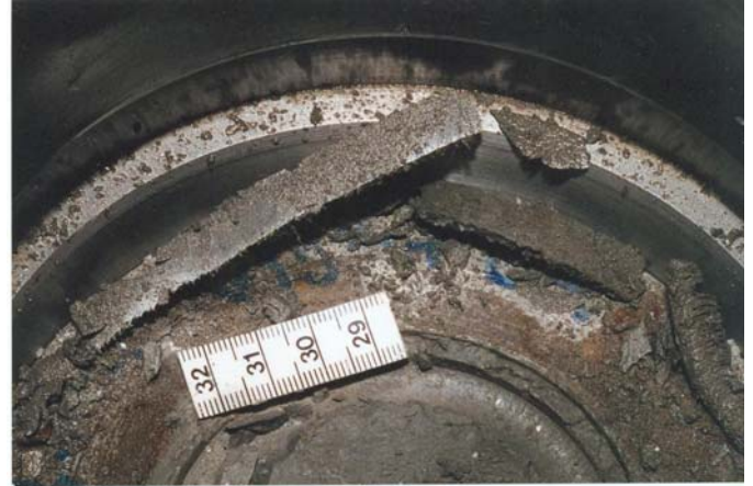
Fig. 5. Saw-toothed ribbon shaped cuttings produced in a single cutter test in mineral oil at 9000 psi 1
