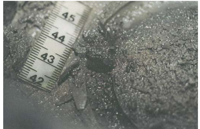
Fig. 22. Test cell of single cutter interference plate test in mineral oil at 9000 psi and 0.006" depth of cut 1
