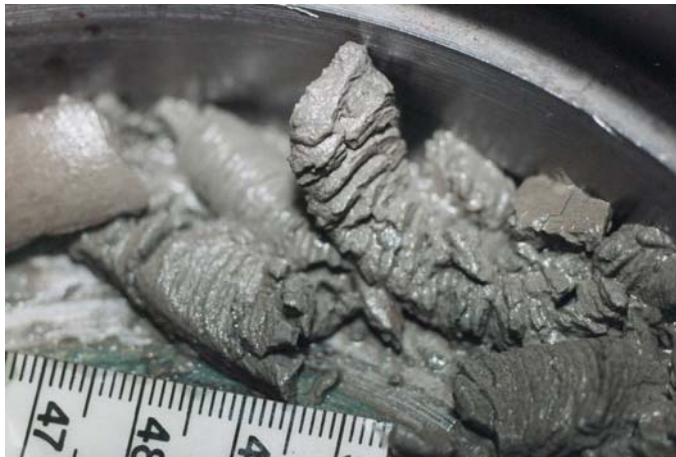
Fig. 4. Saw-toothed ribbon shaped cuttings produced in a single cutter test in water at 9000 psi 1
