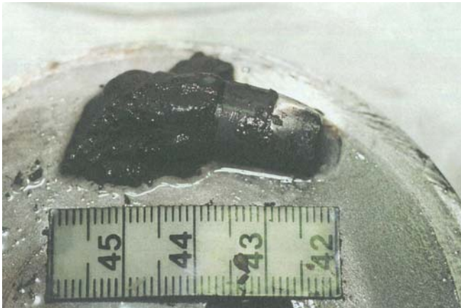
Fig. 12. Global balling in single cutter tests with interference plate in mineral oil at 9000 psi and 0.075" depth of cut 1
