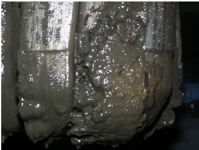
Fig. 2. Global balling in OBM in a full-scale drilling test in Catoosa shale (Courtesy of Baker Hughes)
