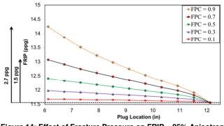
Figure 14: Effect of Fracture Pressure on FRIP – 25% Anisotropy (wellbore is located at 6.125 inches)
