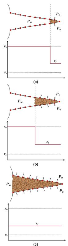
Figure 11: Fracture Plugging; (a) near tip (b) middle of fracture (c) whole fracture
