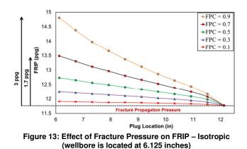
On the other hand, plugging near fracture tip might result in in-sufficient strengthening as shown in Figures (13) and (14). Even with very high FPC; e.g., even 90% reduction in the fracture pressure, increases FRIP by only about 0.5 ppg above fracture propagation pressure or  $\sigma_h$ . These simulations verify that sufficient strengthening cannot be achieved by plugging the fracture at the tip or by simply relying on a tip-screening process.
