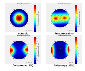
Figure 9: Effect of Anisotropy on Formation Breakdown Pressure
