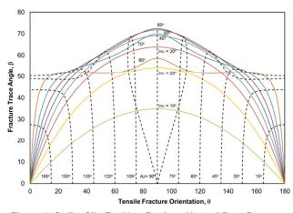
Figure 5: Strike-Slip Faulting Regime, Normal Pore Pressure
