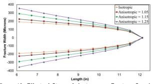
Figure 10: Effect of Stress Anisotropy on Fracture Opening (wellbore is located at 6.125 inches, analysis take into account near wellbore perturbed stress field)
