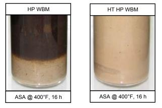
Fig. 1—Comparison of high-performance water-based muds
