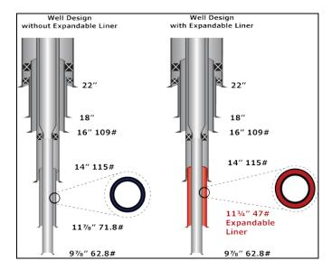
Fig. 2 - Well design defines annular flow area
