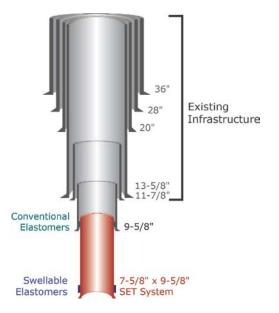
**Fig. 6** - Solid Expandable Shoe Extension Enables Discovery of New Reservoir
