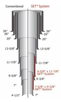
Fig. 5 - Solid Expandable Liners Isolate Depleted Zones
