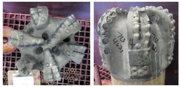
Figure 16: Well A - Second 9.875-in PDC Bit with Six Blades and 16mm Cutters
