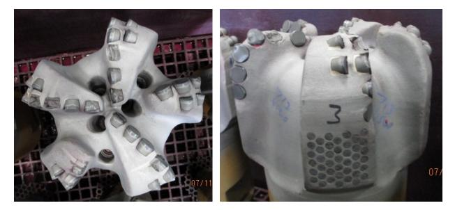
Figure 12: Well A – First 9.875-in PDC Bit with Five Blades and 19mm Cutters
