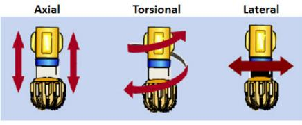
Figure 5: Types of Vibrations: Axial, Torsional and Lateral
