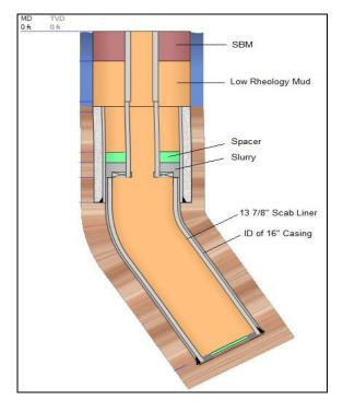
Figure 2: Wellbore schematic with estimated fluid positions after placement
