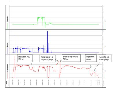
Figure 7: Cement job acquired data (pressure, rate & density)
