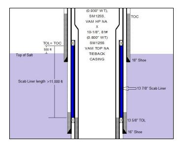
Figure 1: Wellbore Schematic with Scab Liner
