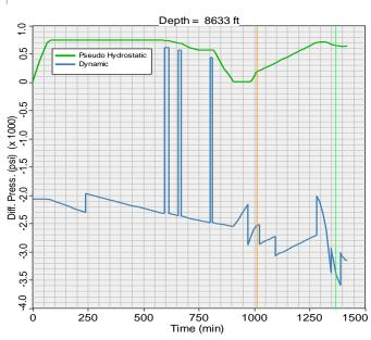
Figure 5: Simulated differential pressure at liner top
