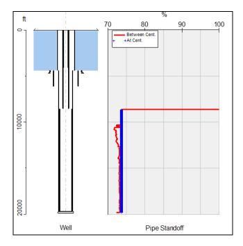
Figure 3: Simulated casing standoff with planned centralizer placement
