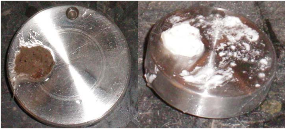
Figure 7 Disks with 1/2 inch holes plugged with ECS-1 combination (left) or reservoir friendly combination (right)
