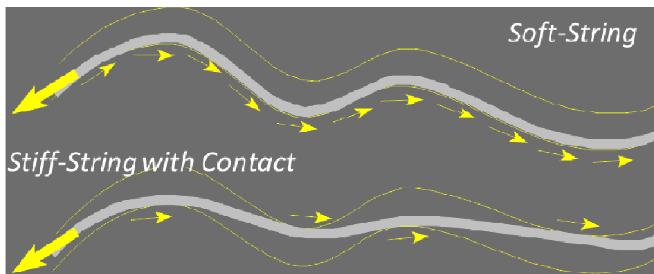
Figure 5: Schematics illustrating modeling difference between Soft-string and Stiff-string model in presence of tortuosity
