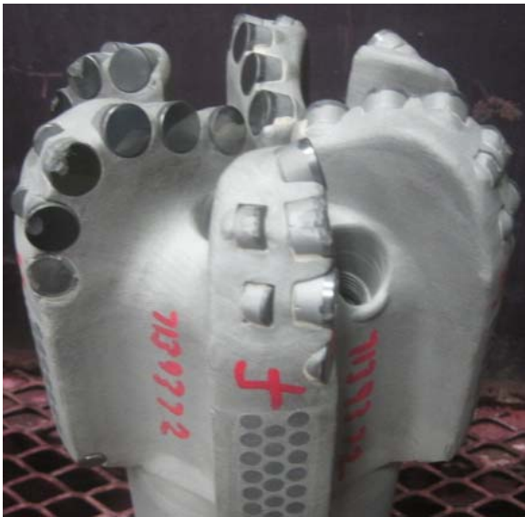
Fig. 17. Bit dull after integrated application-specific features.
