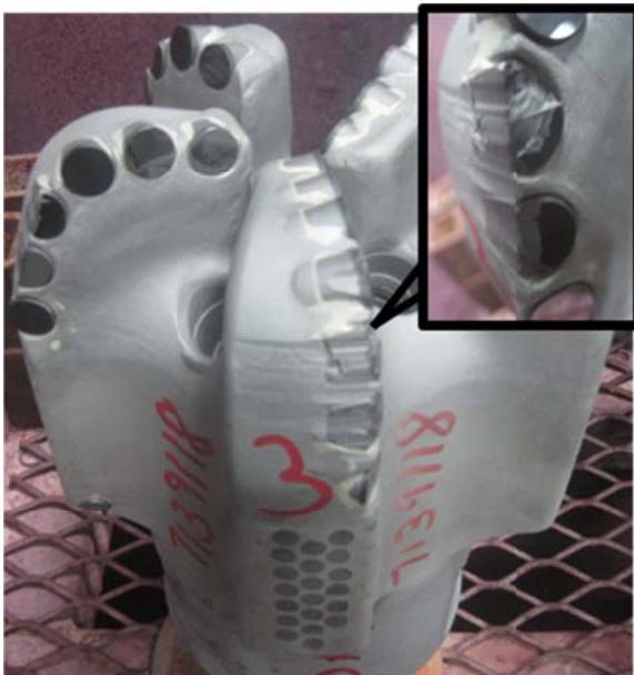
Fig. 15. Initial bit dull for assessment.
