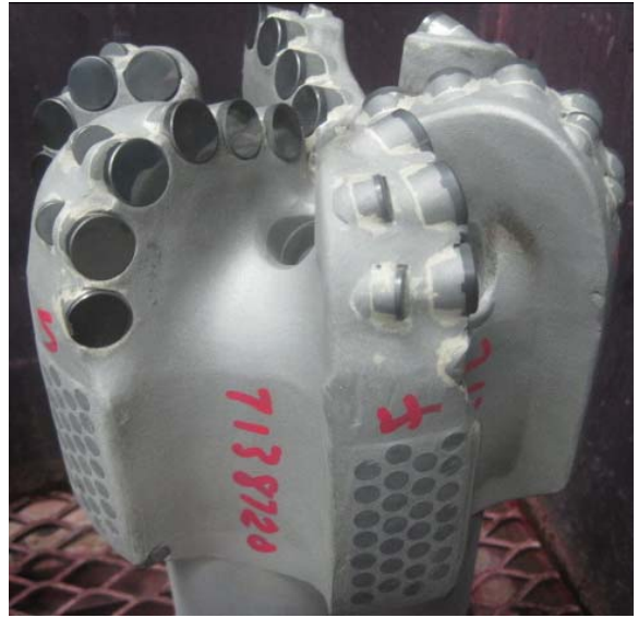
Fig. 18. Bit dull following optimized drilling parameter deployment.
