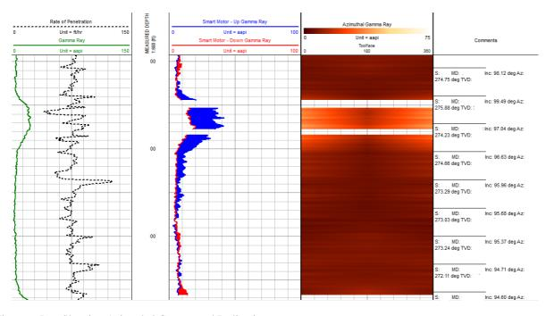
Figure 6: Log Showing Azimuthal Gamma and Inclination measurements
