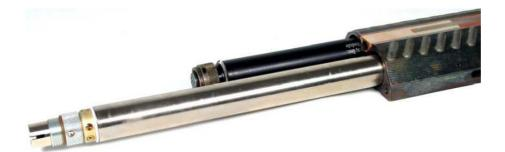
Figure 2: Instrumented motor payload showing telemetry module, sensor module and antenna
