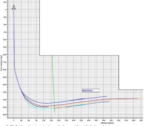
Figure 5: Well plan showing single motherbore with multiple laterals
