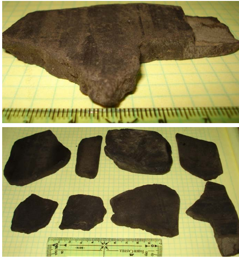
Figure 17. Example of the predominant caving morphology produced during drilling ST1. It can be observed the tabular shape.
