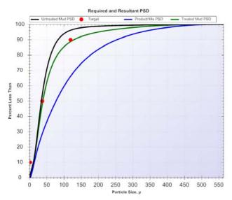
Figure 9: Bridging results with mud PSD
