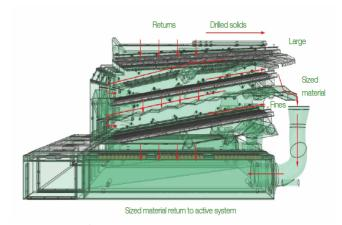
Figure 12: LCM recovery system
