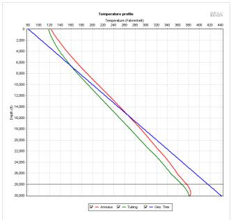
Figure 6: Circulating temperature profile
