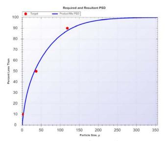
Figure 8: Bridging results w/o mud PSD
