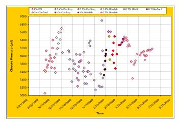
Figure 9: Closure Pressure Responses for Various Clay Inhibition Systems and Concentrations
