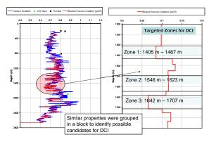
Figure 4: Generated Stress Profile and Potential Injection Targets; Cashiriari 1
