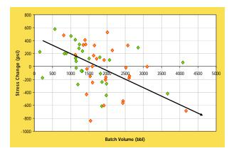
Figure 7: Stress Change vs. Batch Volume
