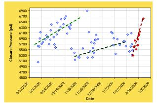
Figure 8: Closure Pressure Monitoring Indicating a Sharp Increase in Slope
