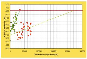
Figure 6: Closure Pressure Responses for Small and Large Injection Batches
