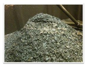
Figure 12 Cuttings after VCS Processing
