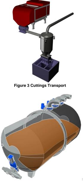
**Figure 4 Vacuum Separation Tank**
