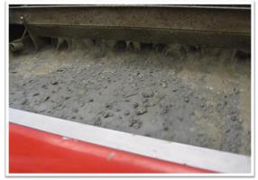
Figure 14 VCS Resisting Blinding
