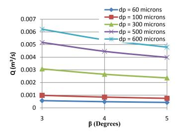
Figure 6: Effect of the tilt angle on volumetric flow rate ( $m^{3}/s$  per meter width of screen) of mud through the screen in the cake section for different particle sizes. The porosity is 0.5.
