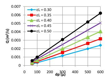
Figure 4: Effect of particle size and porosity on volumetric flow rate (m<sup>3</sup>/s per meter width of screen) through the screen in the cake section. (Note: el = $\varepsilon^L$ ). The tilt angle is 3 degrees.
