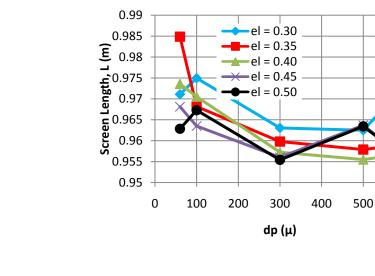
Figure 5: Effect of particle size and porosity on the screen length of the cake section, *L*. (Note:  $el = \varepsilon^{L}$ ). The tilt angle is 3 degrees.
