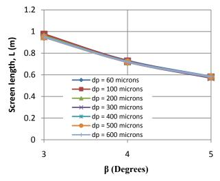
Figure 7: Effect of tilt angle on screen length of the cake section. The porosity is 0.5.
