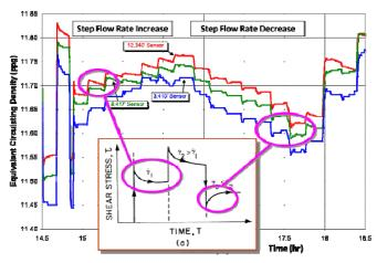
Fig. 4: Impact of flow rate step change on ECD from White et al. (1996) with superimposed Fig. 4.22a from Bourgoyne et al. (1986).
