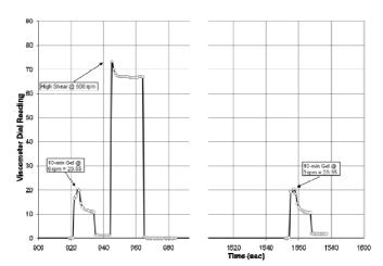
Fig. 3: Test comparing gel-strength measurements at 6 and 3 rpm showing thixotropic effects.
