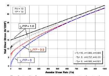
Fig. 5: Annular flow curves comparing exact (markers) and approximate (solid lines) solutions for different R ratios (Zamora and Power 2002).
