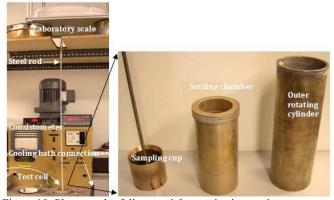
Figure 10: Photograph of direct weight-monitoring equipment
