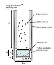
Figure 11: Schematic of direct weight-monitoring equipment.
