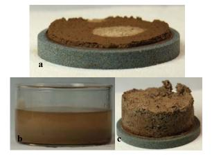
**Fig. 8**. The destructed field-NAF filter cake after the spotting fluid treatment at 500 psid (a), the residual solids on the ceramic disk placed in water showing the wettability (b) and the LCM cake formed after the LCM filtration rate test (c)
