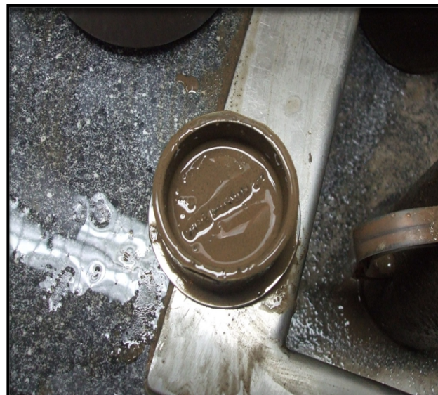
Fig. 4: Photograph of sealed 1500-μm slot.
