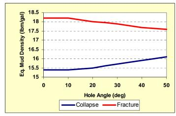
Fig. 1 – A typical safe drilling window up to 50° deviation.
