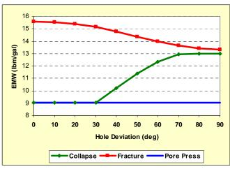
Fig. 2 – Example of a narrow safe drilling window, North Sea ERD well.
