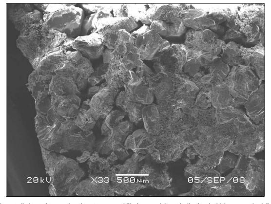
Figure 7. In a lab-controlled test of a core plug, the return permeability increased dramatically after the high-pressure back flush of a mineral oil. It is possible that the short-distance migration of the clay matrix formed larger clayey lumps (center-right) and at the same time cleared some fluid channels (upper and lower).
