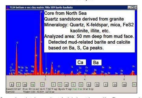
Figure 2. The SEM/EDS can analyze selected areas and spots for their elemental composition. The presence and the intensity of the key elemental peaks are useful in understanding the mineralogy of the core sample and in detecting possible mud invasion.
