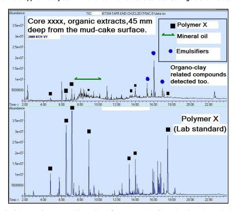
Figure 5. GC/MS analysis of the organics extracted from a North Sea core sample 45 mm deep from the mud-cake surface. Selected ion masses (not shown) are used to ensure the marked peaks match the lab standards.
