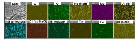
Figure 3. The elemental maps reveal the widespread invasion of the NaBr brine. The carbon map shows the distribution pattern of the organic compounds within core plug.
