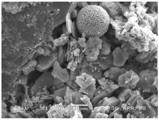
Figure 6. Loosely stacked kaolinite flakes are ready to migrate along with the inter-granular fluids. Fine illite-mica flakes are glued together to form a small lump by organic material (upper right).
