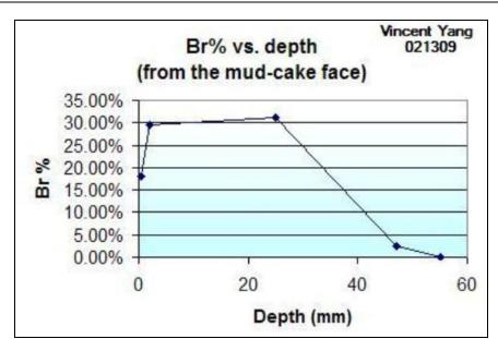
Figure 4. SEM/EDS semi-quantitative analysis of the Br content at different depths of a customer-provided core plug shows that there is a NaBr-invasion zone approximately 30 mm thick under the mud-cake surface. See Figure 3 for the elemental maps.
