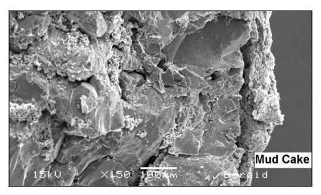
Figure 1. To minimize the possible disruption of the core matrix, the core sample is mechanically opened to expose the fresh cross sections for direct SEM/EDS analyses.
