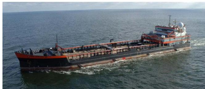
Fig. 11 - At 370 ft, the HOS Centerline was introduced to the deepwater Gulf of Mexico in early 2010 as the world's largest supply vessel. (Photo Courtesy of Hornbeck Offshore).
