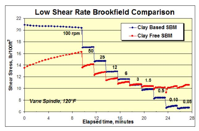
Figure 5 Comparison of ultra low shear readings for clay-based and clay-free SBMs of similar weights.
