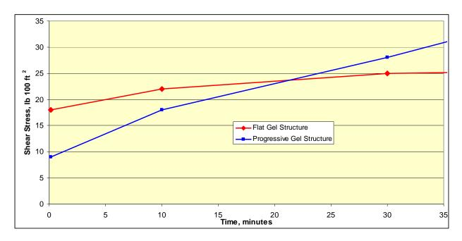
Figure 1 Gel strength development over time: flat gel vs. progressive gel.
