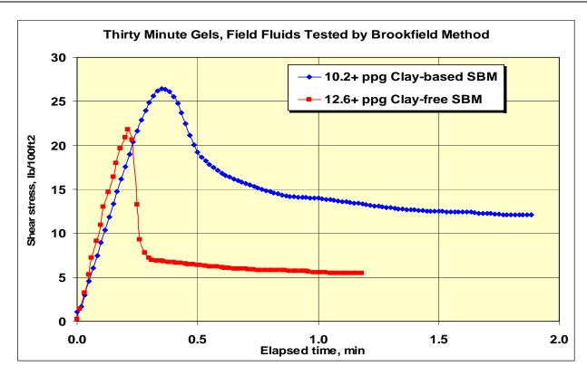
Figure 4 Comparison of shear stress required to break gel strengths built by clay-based and clay-free SBMs.
