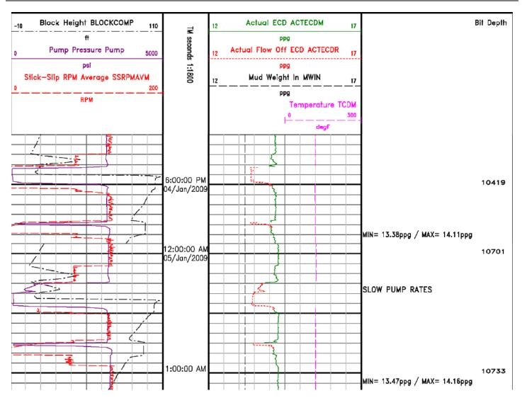
Figure 3 PWD log obtained from Well 2 (clay-free SBM) shows minimal pressure increases after static periods.
