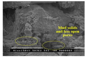
**Figure 6**: CT scan of core plug after circulating NAF DIF and "solids free" NAF DIF
