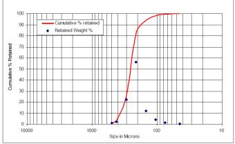
Figure 2: Dry Test Sieve Analysis
