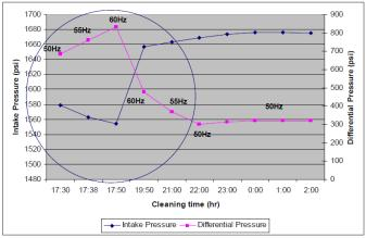
Figure 10: Example of ESP intake and differential pressure
