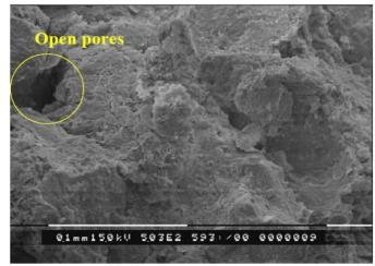
**Figure 5**: CT scan of core plug after circulating NAF DIF
