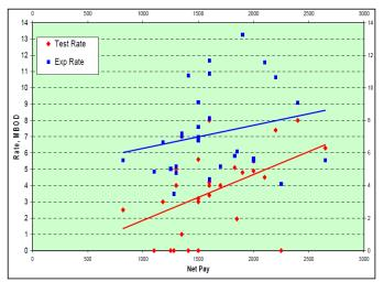
**Figure 8**: Production trends for expected versus actual rate after completing with ICD screen without any treatment
