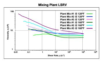
Figure 6: LSRV of plant batch mixes
