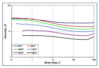
Figure 1: LSRV of a lab prepared IEGPCF
