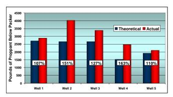
Figure 5: Gravel pack efficiencies of five wells
