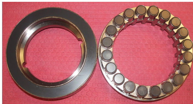
Figure 4. Hydrodynamic Bearing (right) and Rotating Runner (left)
