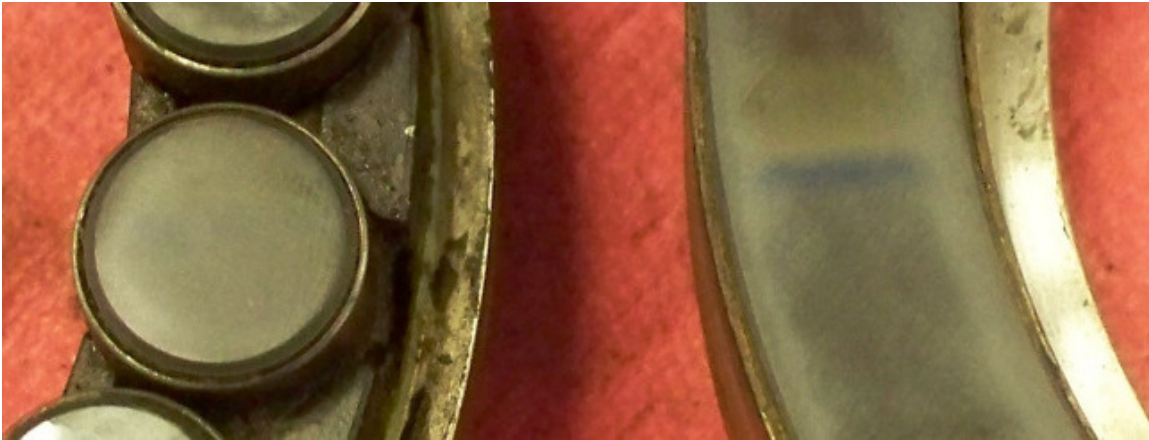
Figure 12. Close-up of Ceramic Components Showing Insignificant Wear
