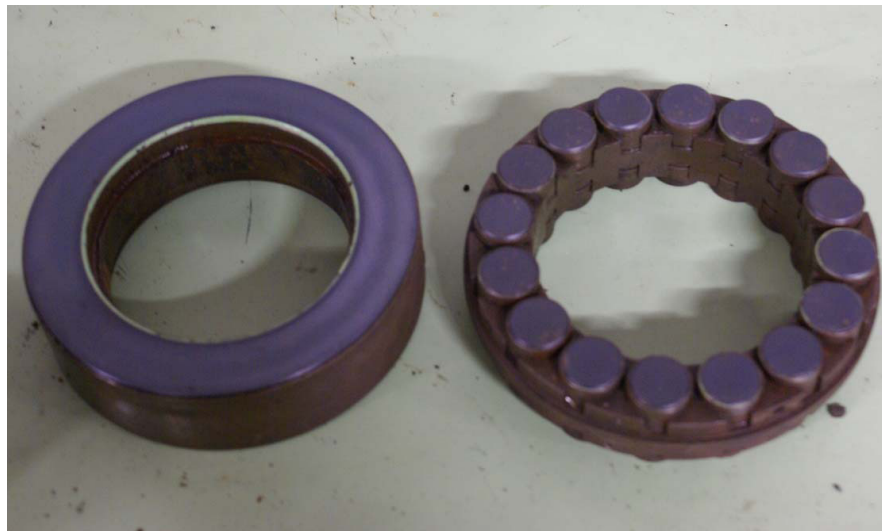
Figure 11. Post Field Operation Picture of Hydrodynamic Bearing (right) and Runner (left)
