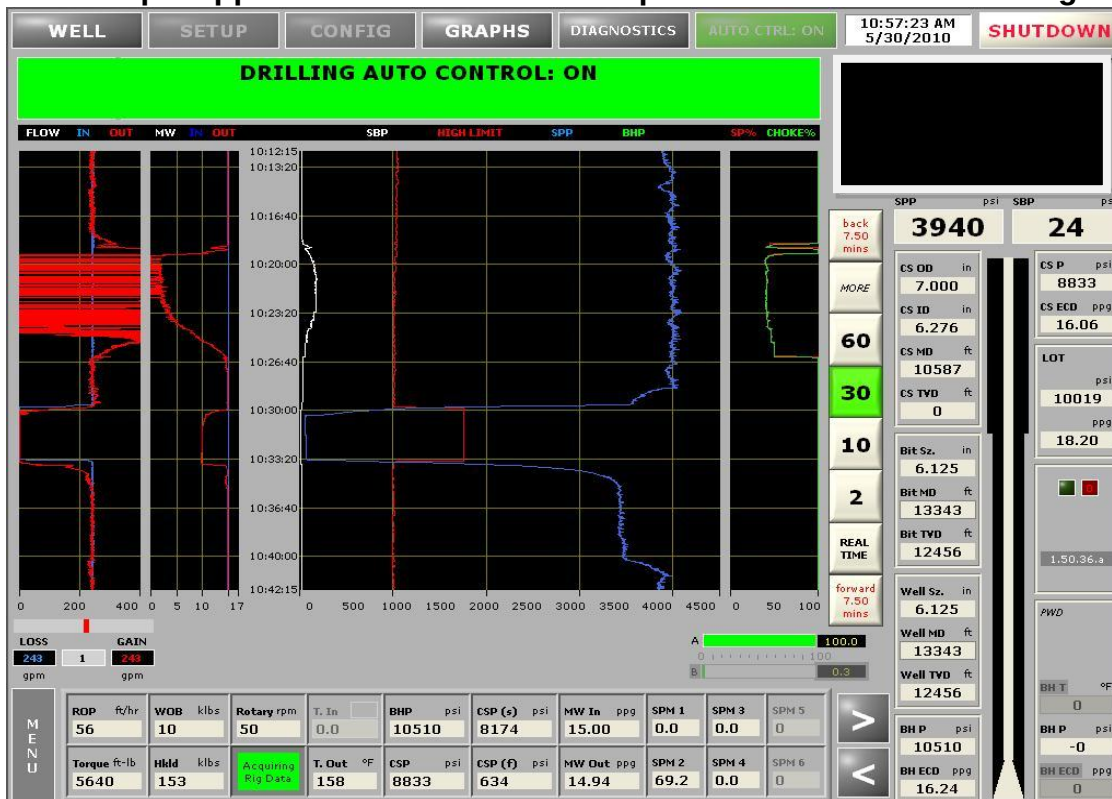
Figure 13: Gas at the surface due to 1 hr rig service, took 6 min. Max gas is 400 unit.
