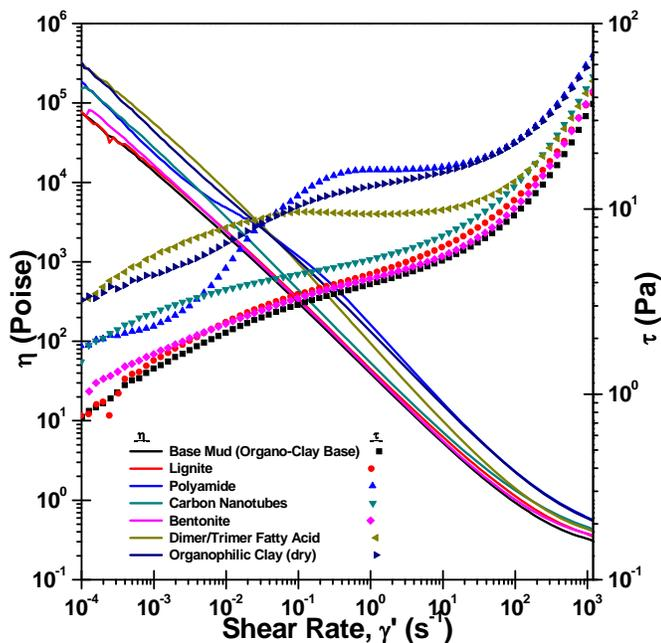
**Figure 3** Flow curves at 120°F using sandblasted parallel plates for the organophilic clay-based invert emulsion mud, OBM #1, with various additives.
