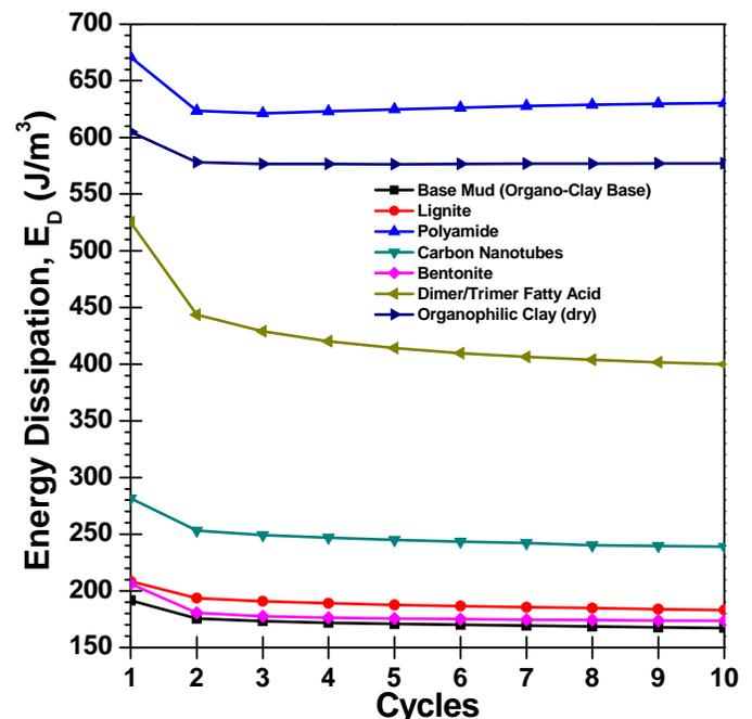
**Figure 8**  $E_D$  from triangular-wave LAOS as a function of oscillation cycle for OBM #1 at 120°F at 0.1-rad/sec and 1000% strain.
