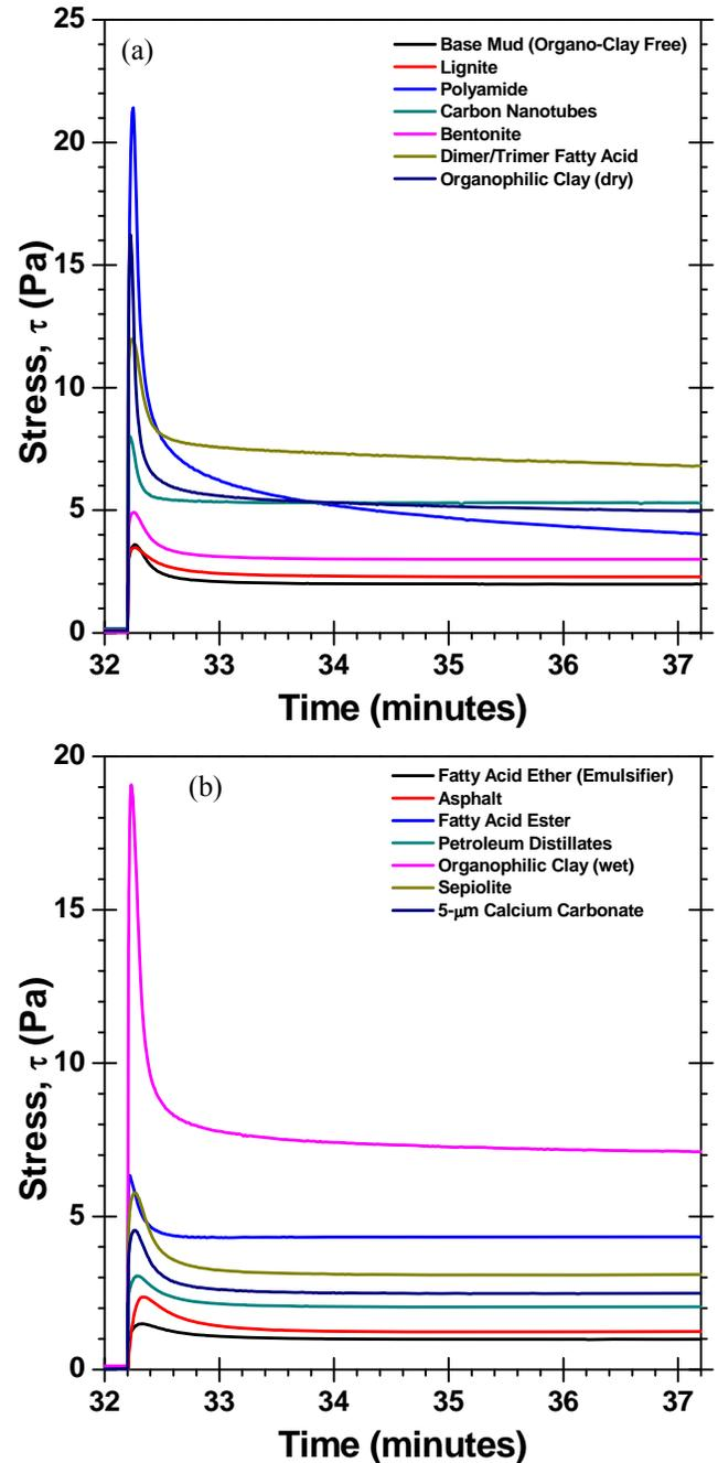
**Figure 6** Gel strength measurements on the MCR501 rheometer for OBM #2 at 120°F after a 10-minute gel period.
