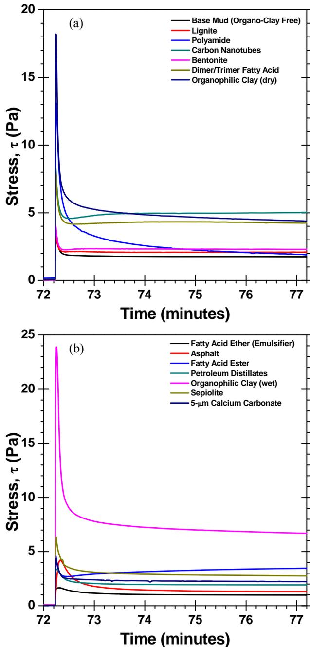
**Figure 7** Gel strength measurements on the MCR501 rheometer for OBM #2 at 120°F after a 10-minute gel period.
