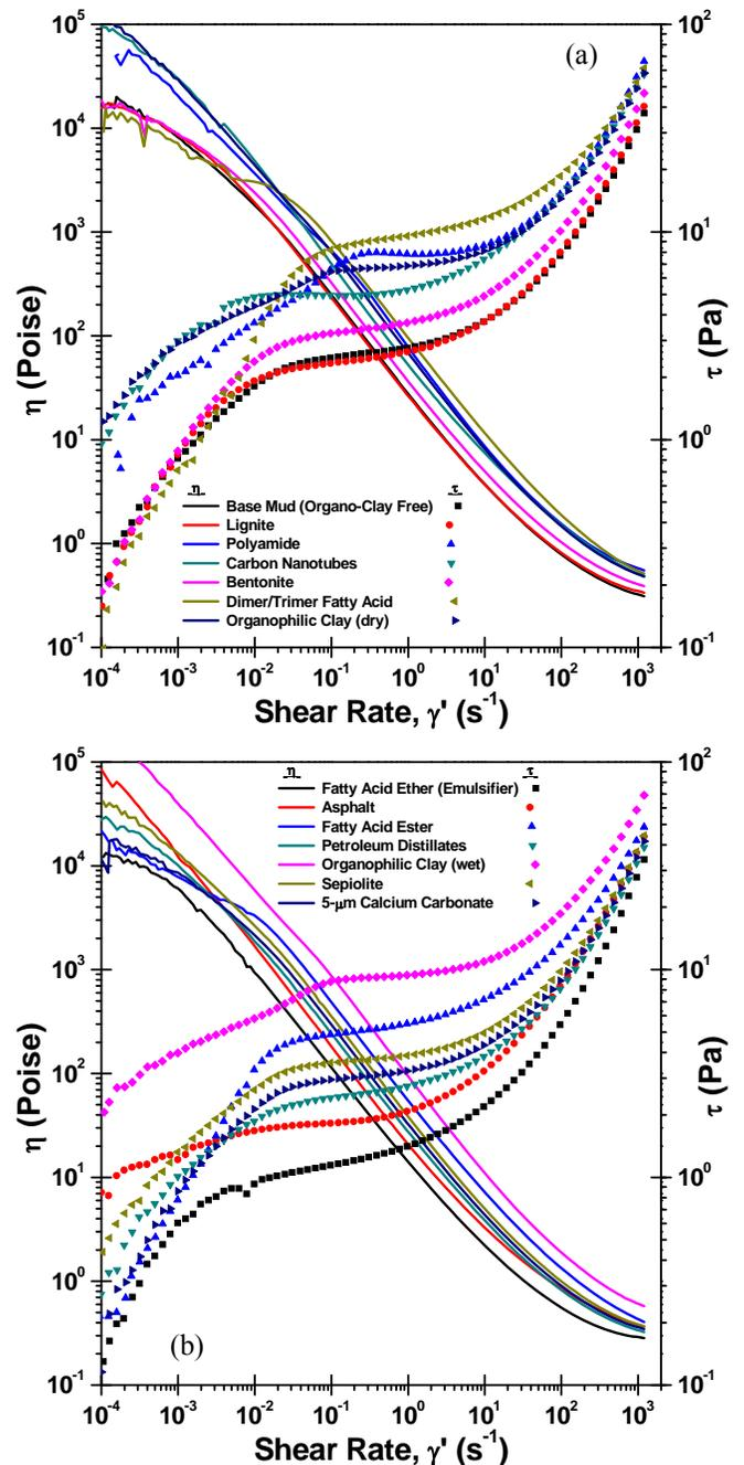
**Figure 4** Flow curves at 120°F using sandblasted parallel plates for the organophilic clay-free invert emulsion mud, OBM #2, with various additives.
