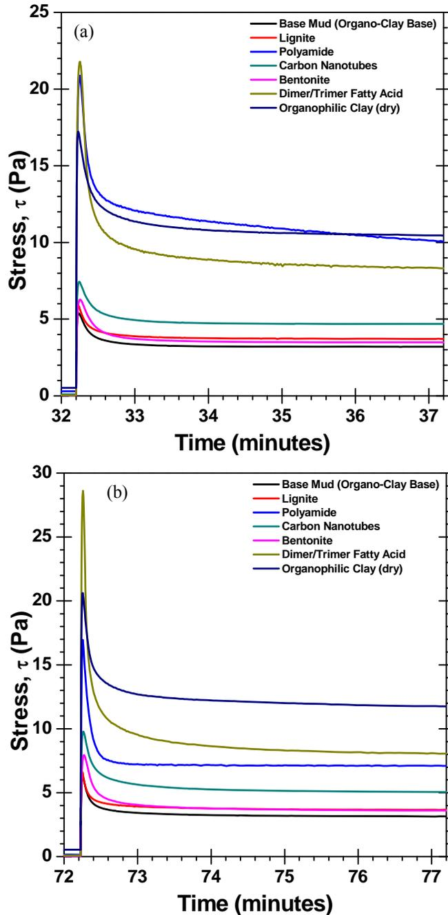
**Figure 5** Gel strength measurements on the MCR501 rheometer for OBM #1 at 120°F after (a) a 10-minute gel period and (b) a 30-minute gel period.
