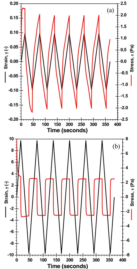
**Figure 1** Triangular-wave LAOS raw data for a drilling fluid sample at (a) 10% and (b) 1000% strain amplitude.
