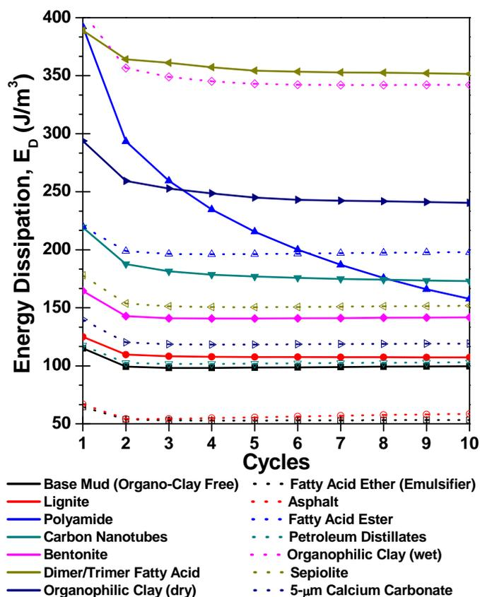
**Figure 9**  $E_D$  from triangular-wave LAOS as a function of oscillation cycle for OBM #2 at 120°F at 0.1-rad/sec and 1000% strain.
