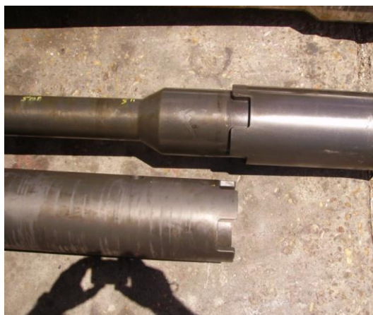
Fig 7 Bottom section of cutaway sub and sleeve featuring splines
