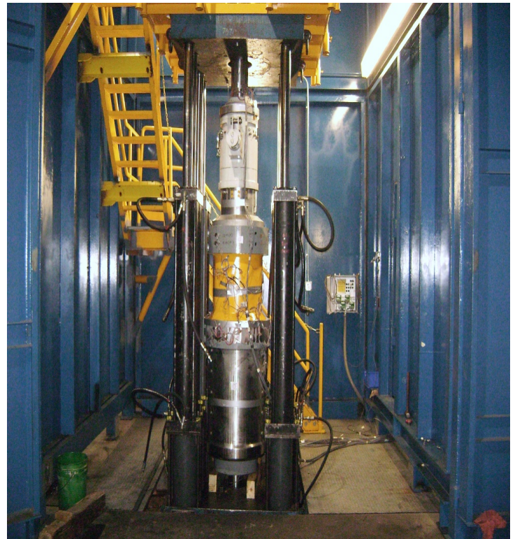
Fig. 1. Ball technology assembly installed in test load frame
