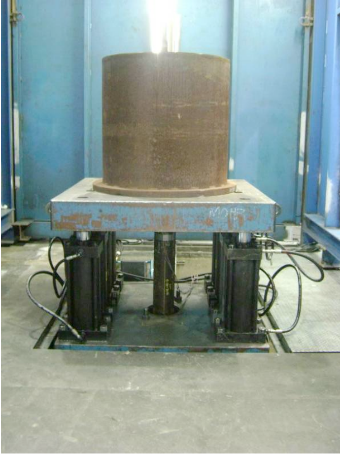
Fig. 5. Conventional slips installed in small load frame
