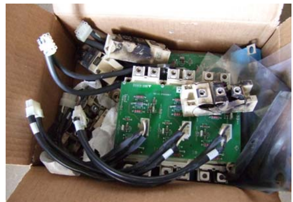
Fig 31 : Damage due to voltage spikes on small to medium powered VFDs. Failure of rectifier devices and DC bus capacitors
