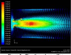
Figure 3 – Flow through an orifice.
