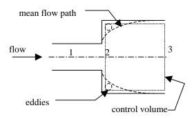
Figure 1 – Flow through an abrupt enlargement.
