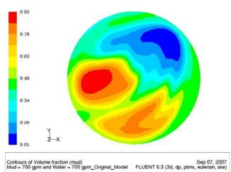
Figure 10 – Later model outlet showing the heavy fluid (red) mixing with the seawater (blue).
