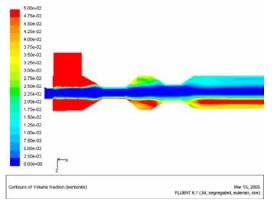
Figure 4 – Vertical cross-section of flow through a mixing table.
