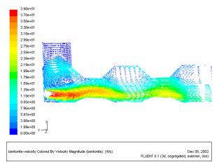
Figure 5 – Vertical cross-section showing velocity vectors.
