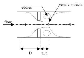
Figure 2 – Flow through an orifice.
