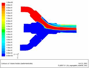
Figure 7 – Early model showing the heavy fluid (shown in red) channeling through seawater (blue).
