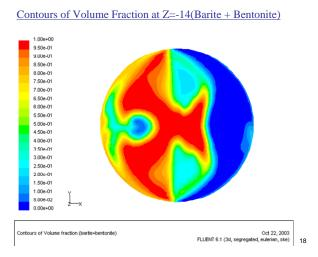
Figure 8 – Cross-section of early model outlet showing the heavy fluid (red) channeling through the seawater (blue).
