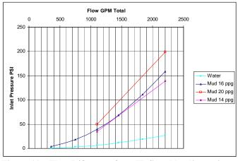
Figure 11 – Flow P/Q curve for a HI-SIDE blending unit.
