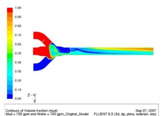
Mud = 700 gpm and Water = 700 'gpm\_original\_Model FLUENT 6.3 (3d, dp, pbns, eulerian, ske) Figure 9 – Later model showing the heavy fluid (red) mixing with the seawater (blue).
