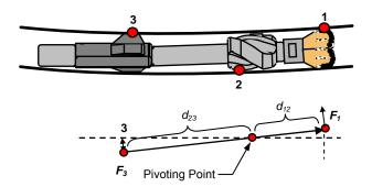
Figure 12: The pivoting point in point-the-bit mode
