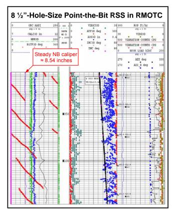
Figure 18: The maximum build rate test with an 8 ½"-hole-size commercial point-the-bit BHA (w/ 98% deflection).
