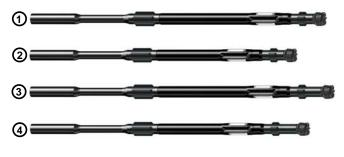
**Figure 14:** Various push-the-bit BHAs tested in RMOTC: 1) Long Push, 2) Short Push, 3) Long Push + Spacer and 4) Short Push + Spacer
