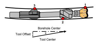
Figure 11: The 2-point-contact geometry in point-the-bit mode
