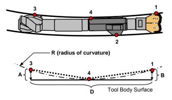
Figure 9: The 3-point-contact geometry in push-the-bit mode
