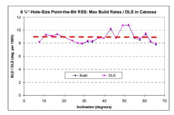
Figure 17: The 8 ¾"-hole-size point-the-bit RSS: Continuous Build-up Test in Catoosa.
