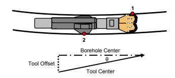
Figure 8: The 2-point-contact geometry in push-the-bit mode
