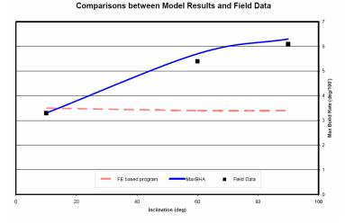
**Figure 7:** Maximum build-rate changes depending on the hole inclination with the third-party 8 ½"-hole-size point-the-bit RSS. (Excerpted from SPE 101186)
