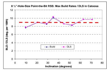
Figure 16: The 8 ½"-hole-size point-the-bit RSS: Continuous Build-up Test in Catoosa.
