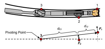
Figure 10: The pivoting point in push-the-bit mode
