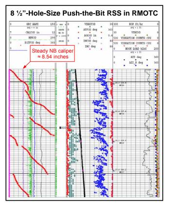
Figure 19: The maximum build rate test with an 8  $\frac{1}{2}$ "-hole-size prototype push-the-bit BHA (w/ 88% deflection).
