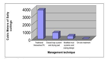
Fig. 1 – Cuttings management can reduce the volume of waste requiring treatment / disposal.
