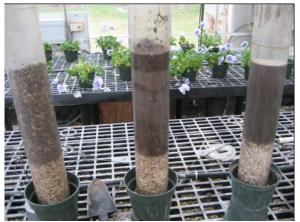
Fig. 2 – From left to right: first tube contains 50% gravel, second contains 50% peat, and third contains 100% cuttings.
