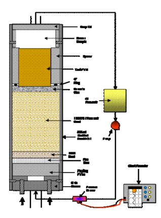
Fig. 9—A Sandpack Permeameter measures the fluids lift off pressure and its damage potential on an Aloxite disc.
