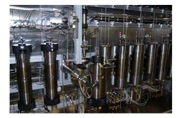
Fig. 12—Schematic of Hassler Cell Permeameter.
