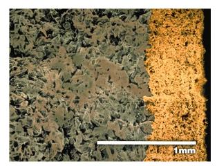
Fig. 5—Sized Calcium Carbonate viewed with an SEM.
