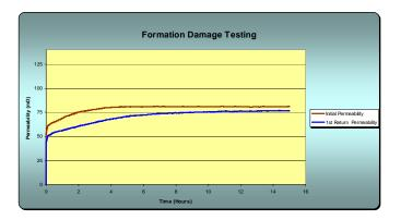
Fig. 14—Filter Cake Destruction by Enzyme Breaker Fluid.
