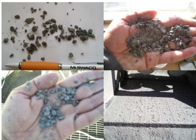
Figure 14 – Images from initial field trial showing high levels of shale inhibition and cuttings quality.
