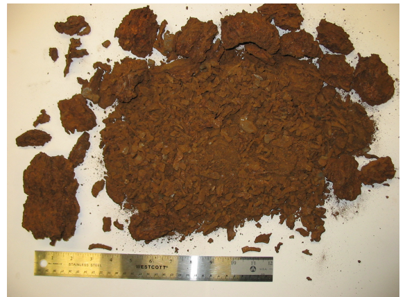
Fig 6 Sample of Debris Removed from the Downhole Debris Filter
