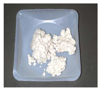
Figure 14. ODP: Internal olefin oil-based oil mud: soda ash water (2:1:4) mixture
