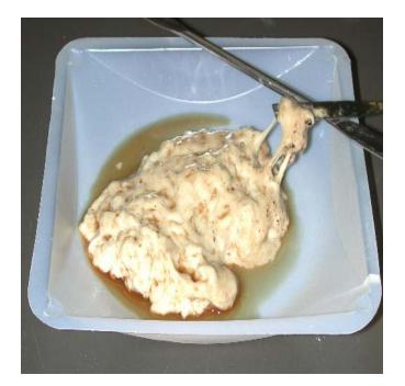
**Figure 15.** The mixture from Figure 14 was hot rolled in 400°F oven for 16 hrs
