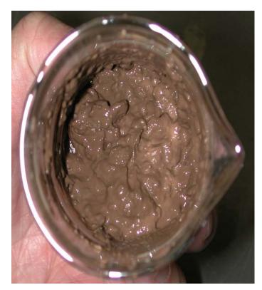
Figure 13. After 1 min. mixing time (AIEP: lignosulfonate mud)(1:20)
