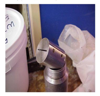
Figure 1. Extrusion rheometer core
