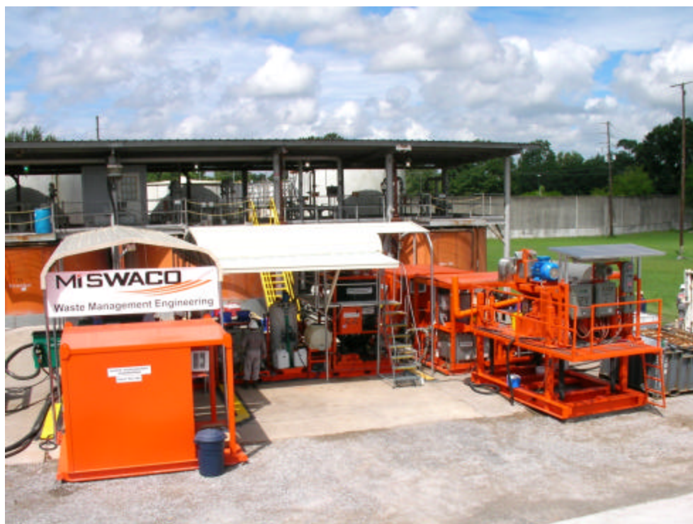
Figure 3 – Pilot-scale unit delivering a 10-gal/min water-treatment flow rate .
