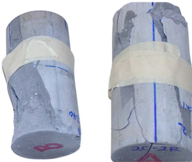
Fig. 11—Cylinder after load-displacement test for Slurry 1.
