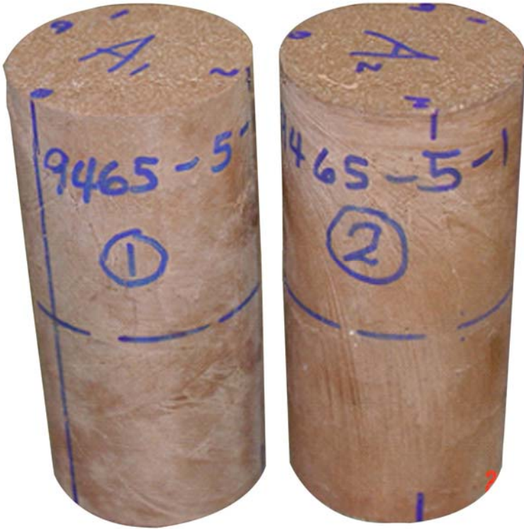
Fig. 12—Cylinder after load-displacement test for Slurry 3.
