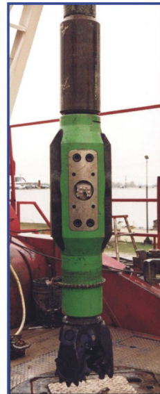
Figure 2—Near-bit reamer cutaway (left) and rigsite deployment (right).
