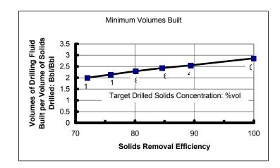
Figure 1 Minimum Volumes required for various Targeted Drilled Solids Concentrations for 35% volume Discarded Solids Concentration
