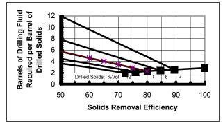
Effect of Targeted Drilled Solids Concentration on Discard Volume Figure 3
