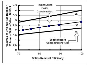
Figure 2 Minimum Volumes required for Various Targeted Drilled Solids Concentrations for 25% volume and 45% voume Discarded Solids Concentration
