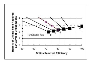
Comparison of Drilling Fluid Volume required with Rule of Thumb of "3" Figure 4
