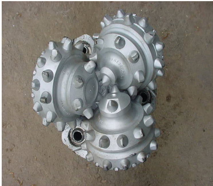
Figure 8. Cleaned bit after the field trial
