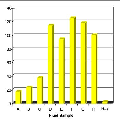
**Figure 7** – Sand bed invasion results for a sized  $CaCO_3$  field mud. Samples A-C were taken from the system before drilling commenced. Samples D-H were taken 12 - 44 hours into drilling and show an approximate 3-fold increase in invasion. The last test (H++) was done with sample H plus 4 ppb of the associative polymer. Vertical scale is sand bed invasion volume x 10 (mL).
