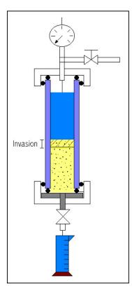
Figure 4 – Diagram of the sand bed invasion test cell. The test is made at 100psi for 30 minutes at room temperature.
