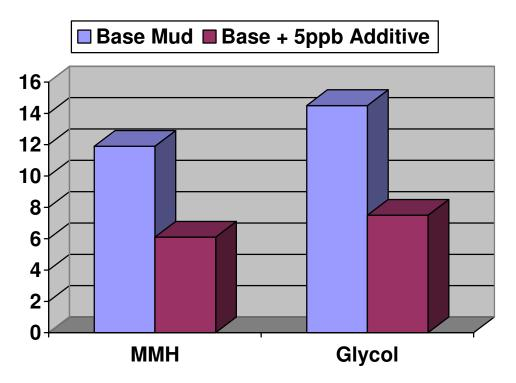
Figure 10 – Differential sticking laboratory test results. Water based muds are at 13ppg. Vertical scale is "sticking index"
