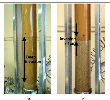
**Figures 5a and 5b** – The left hand figure (a) shows deep Invasion of a field oil-based mud on a 20/40 grade sand bed. The right hand figure (b) shows the same mud with 5ppb of the associative polymer present. The barrier at the sand surface can be seen just below the top arrow.
