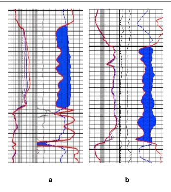
**Figures 11a and 11b** – The left hand figure shows an array induction log of a permeable formation (shaded) drilled with a standard synthetic-based mud. The spaced lines on the left hand side indicate deep filtrate invasion (> 90 inches). The right hand figure (11b) shows an offset well using the same mud but with 5ppb of the micelle-forming additive presence. The overlying lines indicate much less invasion (< 10 inches).
