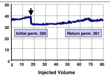
**Figure 9** – Return permeability to brine. Vertical scale is milliDarcies (x10). Fluid is a solids-free water based brine fluid containing 6ppb micelle-forming additive. Core is a synthetic aluminosilicate core. Return permeability = 95%.
