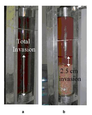
**Figures 6a and 6b** – The left hand figure (a) shows deep invasion of a hematite-weighted 16.5ppg field water-based mud from Colombia on a 20/40 grade sand bed. The right hand figure (b) shows the same mud with 5ppb of the associative polymer present.
