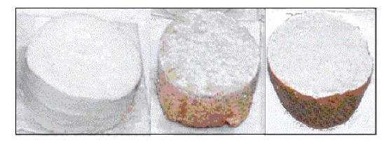
**Figure 2** – A sand bed exposed to different calcium carbonate sizes. From left to right: fine, medium and coarse. If the solids particle size is not appropriate, deep invasion of the solids occurs (left). This can causing severe formation damage and may not effectively prevent mud losses or stuck pipe
