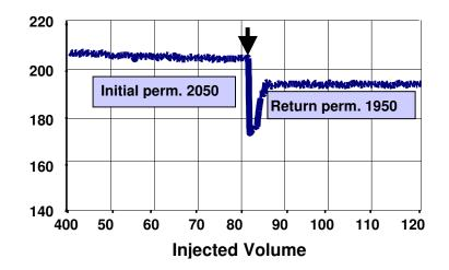
**Figure 8** – Return permeability to brine. Arrow denotes point of injection of associative polymer fluid. Vertical scale is MilliDarcies (x10). Fluid is a bentonite water based mud containing 8ppb micelle-forming additive. Core is a natural sample from a South American well. Return permeability = 93%
