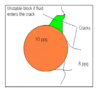
**Figure 1** – The wellbore pressure exceeds the formation pressure by 2ppb. The unstable block is bounded by fractures that will pressurize to the wellbore pressure unless the drilling fluid prevents this. Once pressurized, the block is unsupported by the drilling fluid and is liable to collapse.
