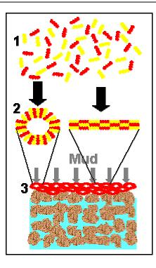
**Figure 3** – A schematic representation of the modified polymers (1) forming "micelles" or assemblages (2) in solution. The assemblages form the low permeability, deformable barrier (3) on the rock surface in the very early stages of mud filtration.
