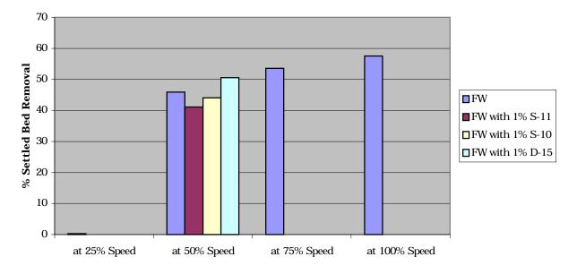
Fig. 1 – Hydraulic shear better than surfactant at removing settled beds.
