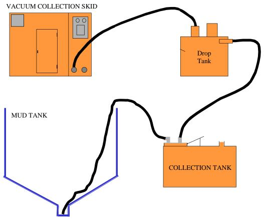
Fig. 2 - Typical Vacuum Collection System in Self-Draining Tank.
