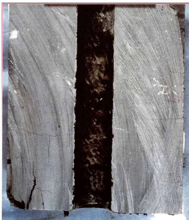
Fig. 2- Pierre shale drilled with KOH lignosulfonate mud and gilsonite G-A at 180°F and 45 hours exposure.
