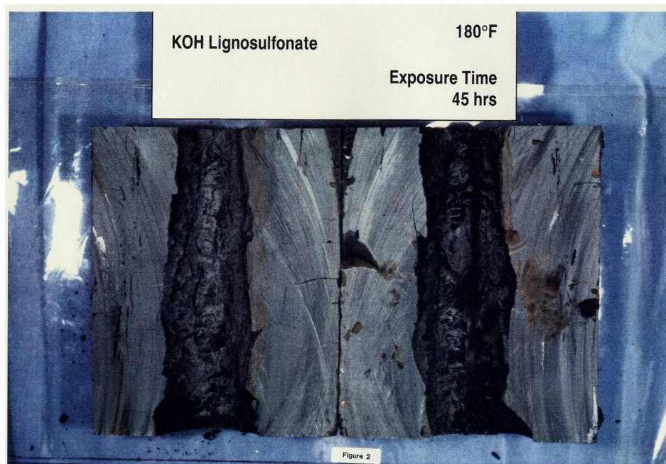
Fig. 1- Pierre shale drilled with KOH lignosulfonate mud after 45 hours exposure at 180°F.
