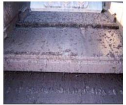
Fig. A8 - Typical cuttings shape and volume on the shaker through Atoka shale.
