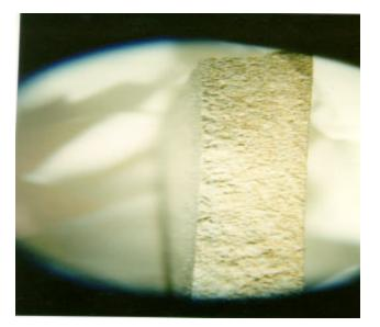
Fig. 4 – Photograph of 10-micron disk on which a filtercake had been deposited from SBM, after addition of a few drops of concentrated sulfuric acid to the exposed broken surface. This result shows the absence of significant invasion of cellulose. Note the similarity in appearance of the two surfaces, especially the lack of any unusual concentration of black spots in the photograph on the right.
