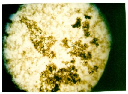
Fig. 2 – Photograph of the test LCM, Highland Glen Fine, after addition of a few drops of concentrated sulfuric acid. Note the dark color of the fluid and the black residue.
