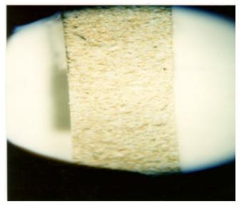
Fig. 3 – Overview photograph of the 10-micron control disk (before filtercake was deposited) and addition of a few drops of concentrated sulfuric acid to the exposed broken surface. Note the absence of any dark color other than at the surface. The black deposit on the surface of the control disk (upper left) resulted from contact of the acid with some facial tissue that was adhering to the surface.
