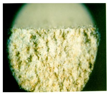
Fig. 6 – Detail of the 10-micron disk after filtercake buildup.
