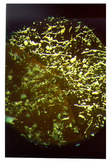
Fig. 7 - Photomicrograph of Highland Glen Fine after two hours of soaking in water. The water is bounded by the brown line, with water being on the left. Note the similarity in particle shape and size in the two zones.
