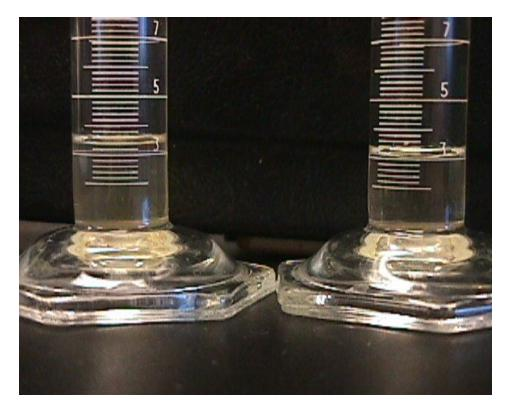
Fig. 1 – Photograph of the effluents from cake formation on the 5-micron and 10-micron disks, illuminated on four sides by very bright point sources of light. Note the absence of bright spots in the fluid, indicating the absence of particulate matter.
