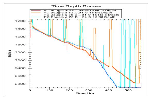
Figure 4. Bougie time depth curves: RSS (blue) versus motors (red).
