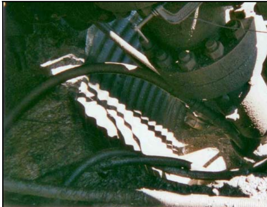
Fig. 8. Parasite string exiting the wellhead.
